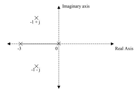
**Step 4:** The number of root locus branches equals the number of open-loop poles. Therefore in this case, the number of root locus branches is equal to 4.
