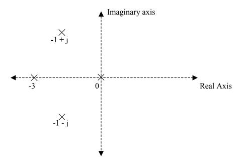
**Step 2:** Each branch of the root locus originates from the open-loop pole at K = 0, and terminates at  $K = \infty$ , either on an open-loop zero or infinity. Since the system given does not have any zero, all the branches terminate at infinity.
