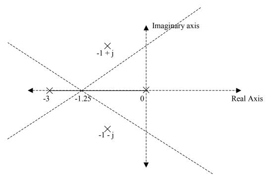
Step 6: The breakaway points of the root locus are determined from the roots of the equation  $\frac{dK}{ds} = 0$ .
