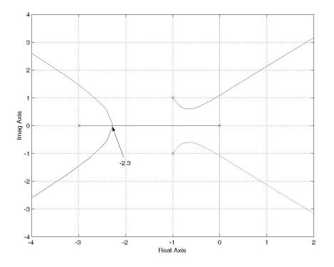
To determine the value of *K* at which the root locus cuts the imaginary axis
