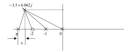
$-\theta_p - 112.41 - 120 + 103.898$ . This angle must be equal to -180 degrees. Hence the angle subtended by the compensator pole with the closed loop pole is 51.488 degrees.
