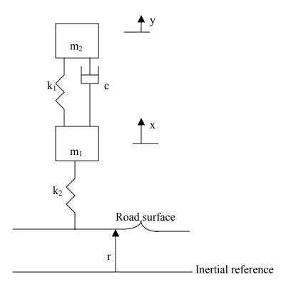
The system shown below is an approximation of a suspension model for one wheel of an automobile. The displacements of the masses, 'x' and 'y' are from their equilibrium positions.
