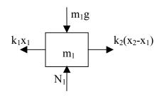
Writing the Newton's second law of motion, which states that the sum of the forces acting on the body must be equal to the product of its mass and acceleration.
