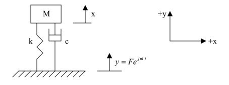
Notice that, the base of the system moves by 'y' units independent of the mass. But in this case, we however know how the base moves, as given by the harmonic function. So in effect this is just a one degree of freedom problem. That is in other words, there are two degrees of freedom for this system, but out of which one degree of freedom is known.
