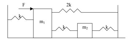
2) For the system shown below, derive the governing differential equation of motion.
