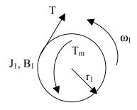
where  $J_1$  is the inertial of the motor,  $B_1$  is the motor damping constant,  $T_m$  is the torque developed by the motor, T is the tension in the string.
