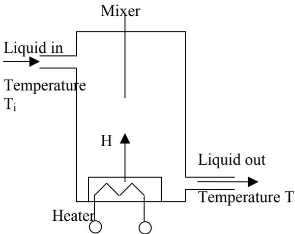
Assume that the tank is thermally insulated and the liquid in the tank is kept at uniform temperature by perfect mixing with the help of a mixer. Assume that the steady state temperature of the incoming fluid is  $T_i$  and that of the out flowing liquid is  $T$ . The steady state thermal input rate from the heater is  $H$  and the liquid flow rate is assumed to be constant.
