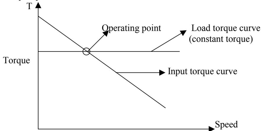
Torque-speed curve of a DC motor
