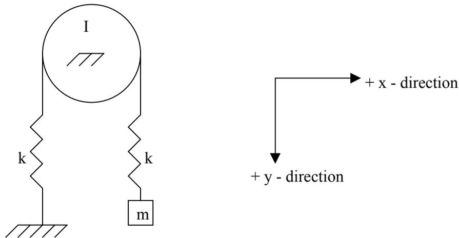
The Disc with mass moment of inertia ‘ $I$ ’ rotates in the counterclockwise direction. The block of mass ‘ $m$ ’ moves a distance of ‘ $y$ ’ units from the static equilibrium position in the positive  $y$ -direction.
