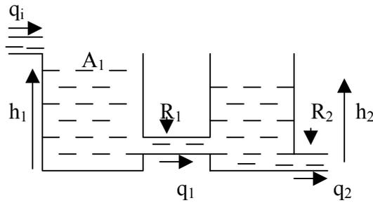
The above figure represents a two-tank liquid level system.
