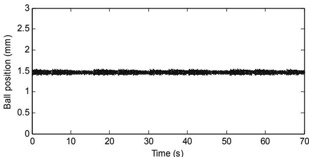
Fig. 3. NCS test bed response with a control loop closed over the Ethernet.
