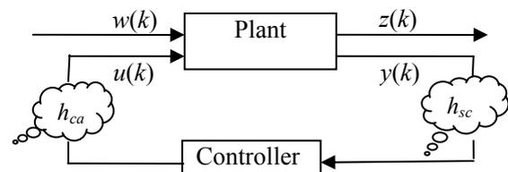
Fig. 1. An NCS with network-induced time delays.
