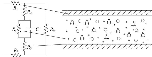
Fig. 5. IPMC structure and the corresponding RC system.
