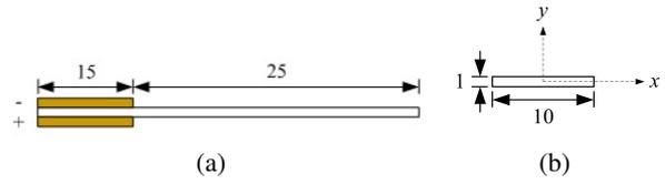
Fig. 1. Dimension of our IPMC strip (units: mm).
