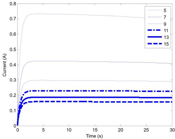
Fig. 7. Simulation of current with various surface conductivities of a thick IPMC strip.
